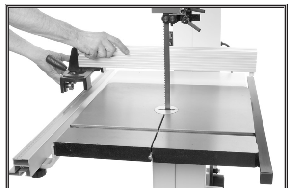
Figure 16. Installing fence onto rails.
